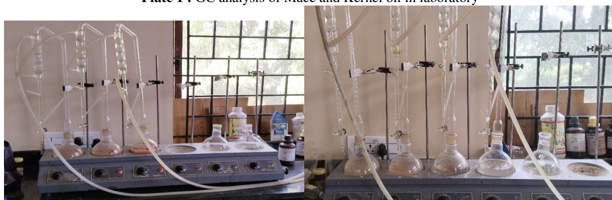
Plate 2 : Volatile oil extraction of Mace and Kernel in laboratory
