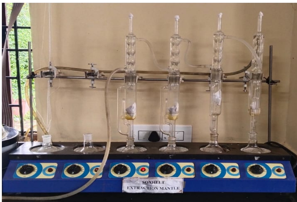
Plate 3 : Oleoresin extraction of Kernel in laboratory
